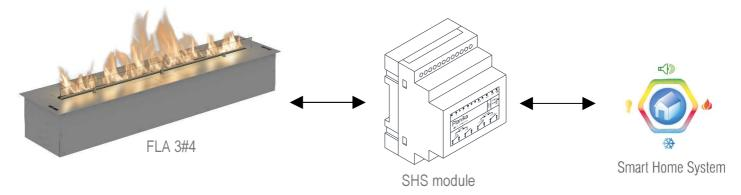
SHS module enables following control options: switching the device on and off and adjusting flame size.
