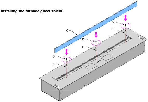
Situations where the installation of glass shield protecting the furnace is necessary.
