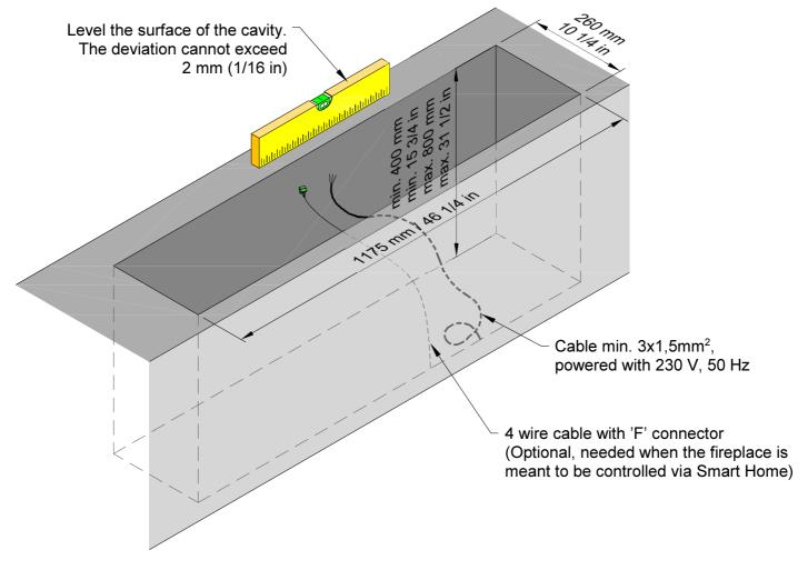
Place the external tank 'B' in the cavity.
