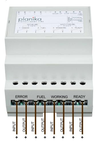
INPUT – voltage signal input, from 12V to 24V DC OUTPUT – voltage signal output, from 12V to 24V DC
