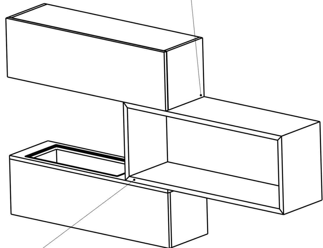
Middle and lower unit connected by screws/bolts which are hidden inside the lower unit
